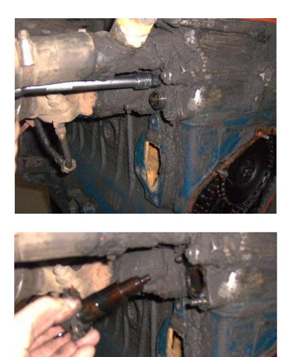
Use the 13mm long socket to remove the crankcase ventilation system cover complete with the oil dipstick and vent hoses. That big hose is supposed to go to the air filter, but this engine had so much blow-by that it kept fouling the carb with oil so I opted by letting it discharge to open air:
