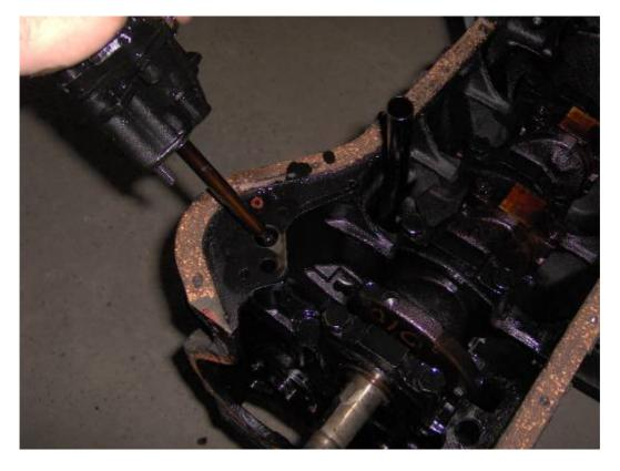
In this position the crankcase vent system return tube is easily removed:
