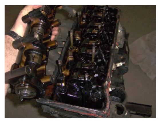
The cylinder head bolts can be very tough to remove, so use a 19mm socket along with an extension and a big cheater bar to persuade them:
