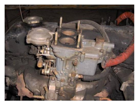
Use the 13mm combination spanner to remove the four 8mm nuts that hold the carburetor to the intake manifold:
