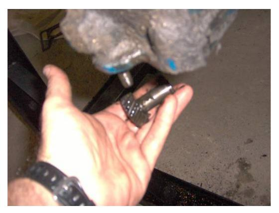
Use the 13mm socket to loosen the oil pump bolts and finally remove the pump:
