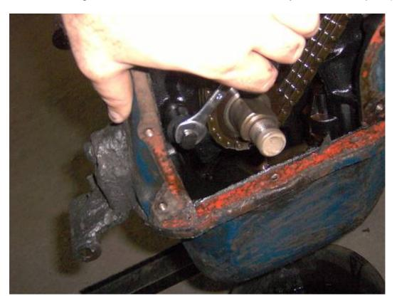
Undo the tensioner shoe fastening bolt with a 17mm socket and remove the shoe:
