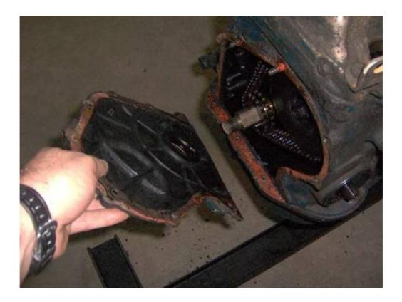
A quick look inside reveals: the crankshaft (1) and oil pump/distributor drive (2) sprockets, the timing chain itself (3), the chain limiting pin (4) and the tensioner shoe fastening bolt (5):
