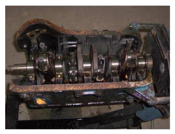
...Followed by the thrust half-rings which limit the crankshaft endplay. There's one on each side of the No. 5 main journal:
