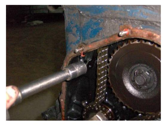
Use a screwdriver to lock the chain and use the 17mm socket to loosen both the camshaft and oil pump drive sprocket bolts, but don't drive them out all the way:
