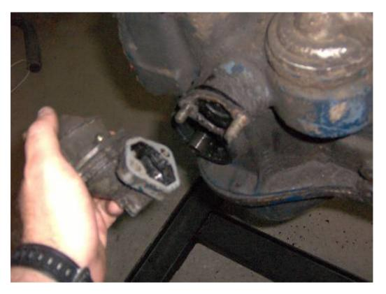
Use a screwdriver to pry loose and finally remove the timing chain cover. Look at all that nasty sealant my old mechanic used:
