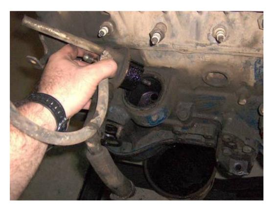
Both the camshaft and oil pump drive sprockets have these special lock washers to keep their bolts from coming loose. Use a cold chisel and tap with a hammer to unfold the washers and expose the bolts:
