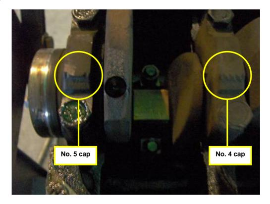
Connecting rods are also marked, but in this case matching numbers are used:
