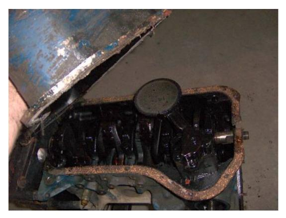
Oh, once the block is inverted, the distributor drive gear should fall by itself...
