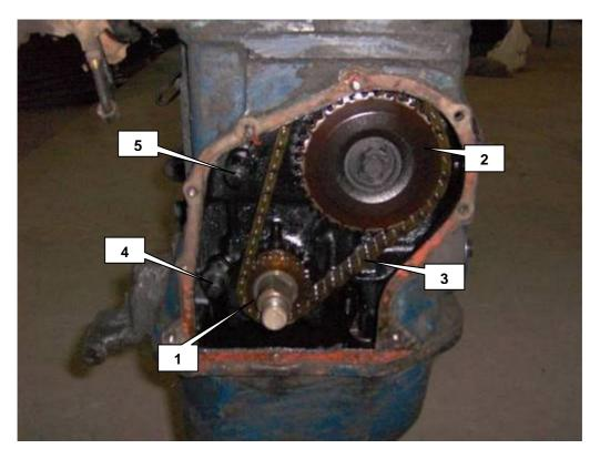
Different manufactures use different tensioner nut dimensions. So far l've seen having 12mm, 13mm and 9/16" heads. Mine had a 13mm nut:
