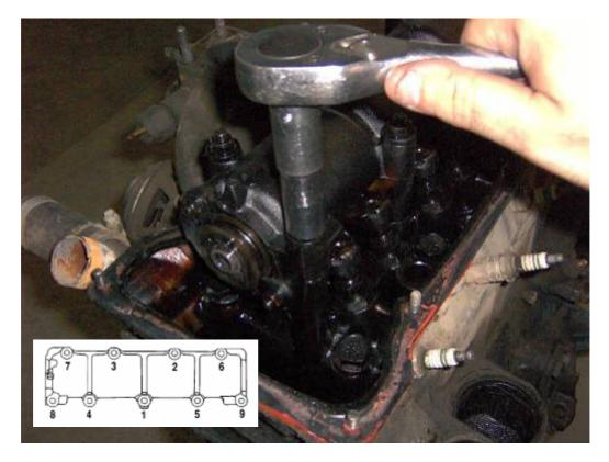
After which the bearing assembly can simply be lifted out, exposing the valve rockers:
