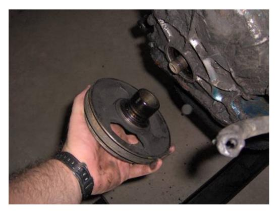
While taking the pulley off I found out I didn't remove the rear crankshaft seal holder before bolting the engine to the stand, so used a 10mm socket on the 3/8" ratchet and a flat screwdriver to pry on the holder:
