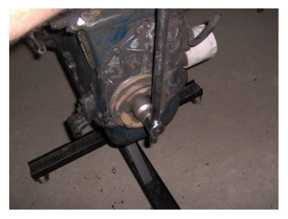
...Once the nut is removed, out comes the pulley...
