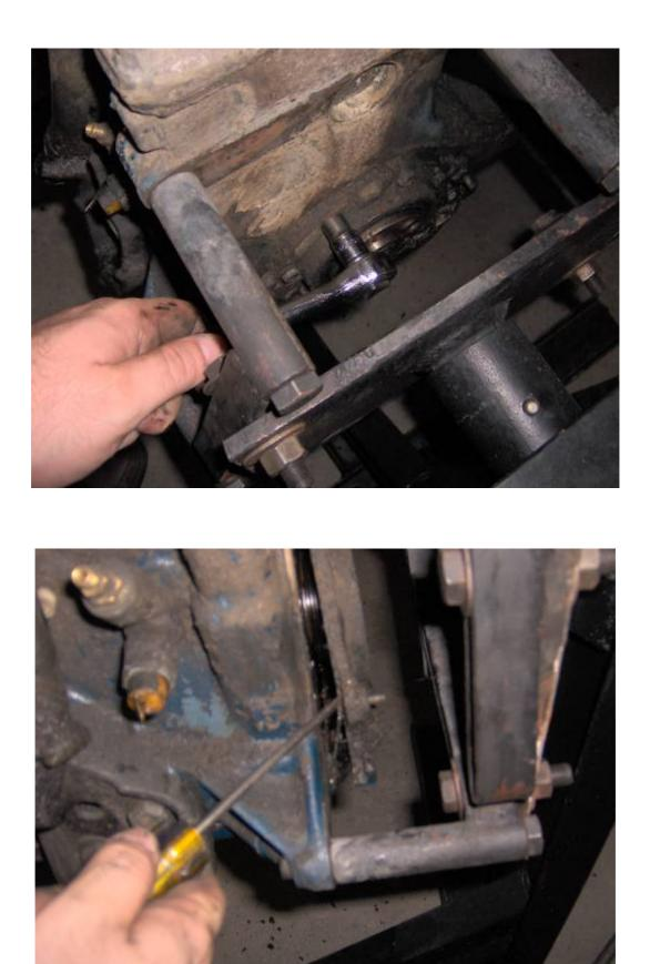
Use the same 10mm socket (and a 13mm one) to remove the nuts and bolts of the timing chain cover:
