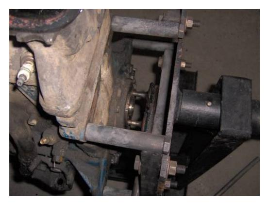
...While cracking the crankshaft pulley nut with the 1  $\frac{1}{2}$ " / 38 mm socket and a big cheater bar. That damn nut was so tight I actually had to stand with both feet on the stand (how redundant!) to prevent it from tipping over...
