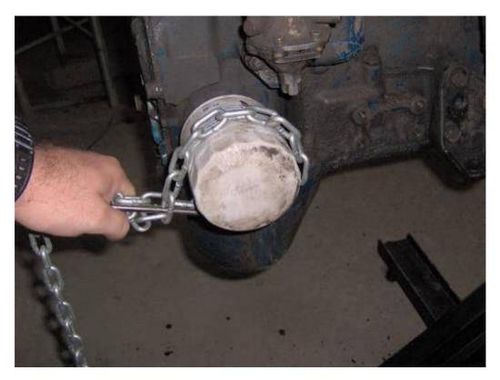
The fuel pump was in the way too, so took it off with the help of a 13mm socket:
