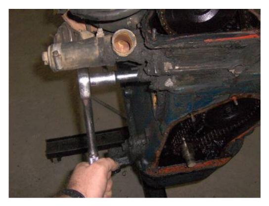
Use the 10mm socket to remove the tensioner fastening nuts before pulling it off the block:
