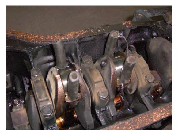
Use a 17mm socket to loosen the main bearing cap bolts and remove all of the caps:
