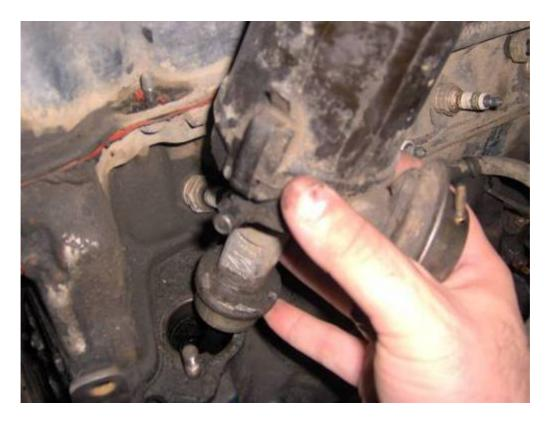
Loosen the bolts that hold the fan and its drive pulley to the water pump hub with a 13mm socket and remove the fan/pulley. As you can see, my engine has no fan shroud:
