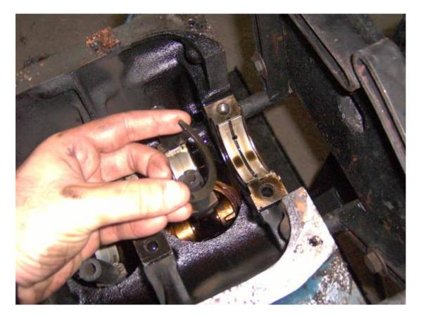
The piston-connecting rod group can now be pulled out from the block (engine inverted in picture)...
