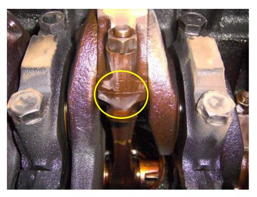
A 14mm or 9/16" socket is required to remove the connecting rod cap nuts:
