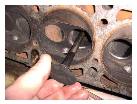
...And finally remove the old valve stem seals. If the guides/valves are still in good condition and are going to be reused, take special care not to damage the guides while removing the seals:
