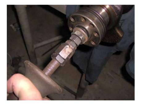
A couple hits of the 5-pound slide hammer are fair enough to pull the pilot bearing out from the crankshaft's rear end...
