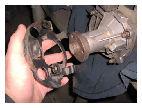
...And finally remove the pump's front housing:
