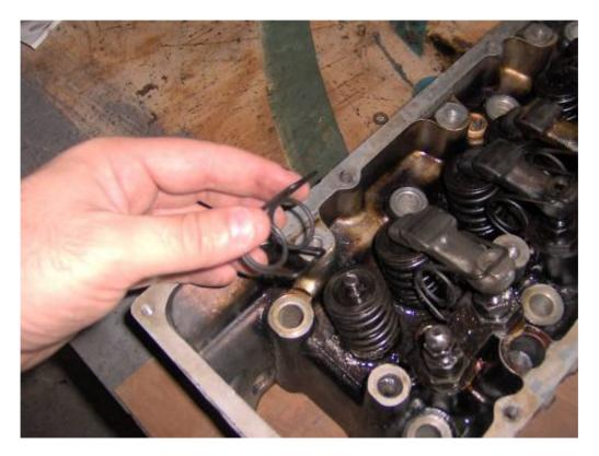
The adjusting screws should be removed from their threaded bushings. These screws can be very hard to remove on old engines, so it's a good idea to spray them with some penetrating oil (such as WD-40) and let it sit overnight:
