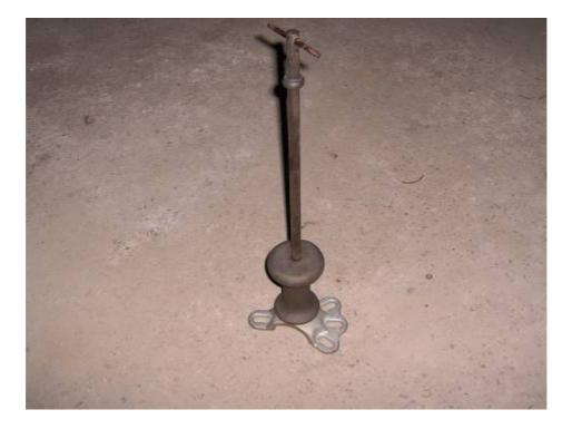
The puller flange and slide hammer shaft have 5/8" UNF threads, so it was pretty easy for me to fabricate a simple pulling fixture using a 5/8" UNF long nut, a standard  $\frac{1}{2}"$  grade-8 nut/bolt and a flat  $\frac{1}{2}"$  washer. I had the  $\frac{1}{2}"$  bolt head turned up in the lathe until its diameter was a tad smaller than the pilot bearing's inner race and *Voila!* Now I had something that can be used as some sort of hook on the end of the slide hammer:
