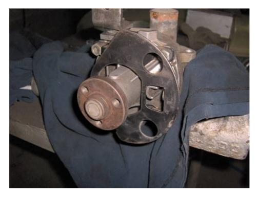
...Then, using a long 13mm socket and ratchet, remove the four fastening nuts:
