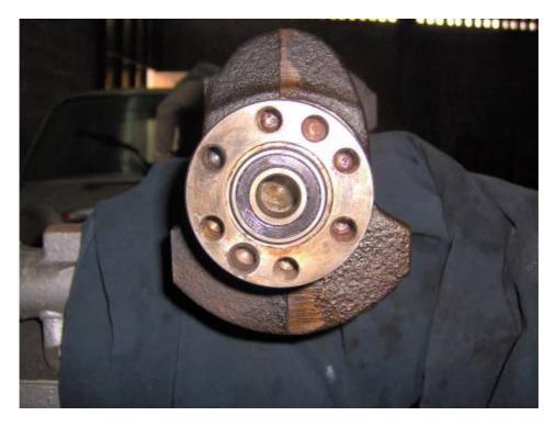
There are a good number of tricks for removing a pilot bearing, but I feel the easiest way is by using a slide hammer along with a proper pulling fixture. I happen to have a K-D Tools axle shaft puller which proved extremely effective for this purpose:
