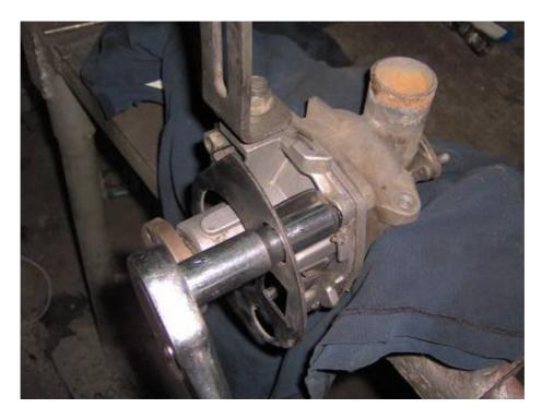
Remove the fan shroud bracket:
