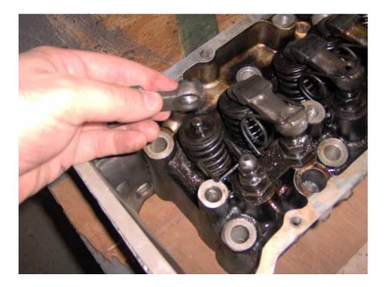
After removing the rocker, the rocker spring can now be easily pulled out from its hook under the adjusting screw:
