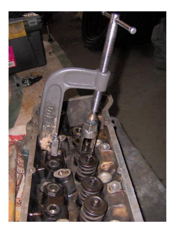
Luckily for me, the valve adjusting screws have M12 x 1.25 threads. If this wasn't the case, I seriously don't know how I would've managed to engineer things out:
