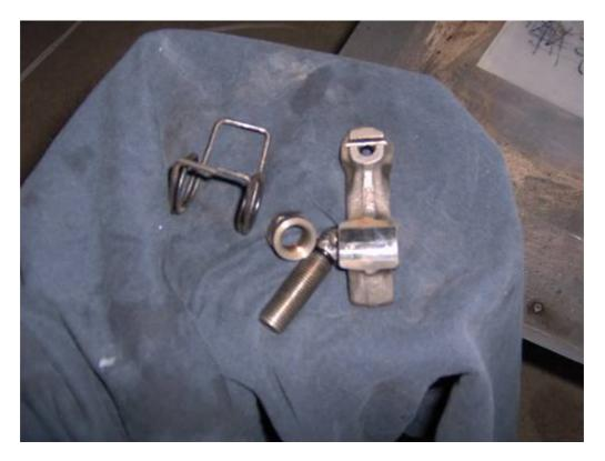
...And finally place them in separate transparent plastic bags, which have been previously marked with a permanent marker according to their position on the cylinder head:
