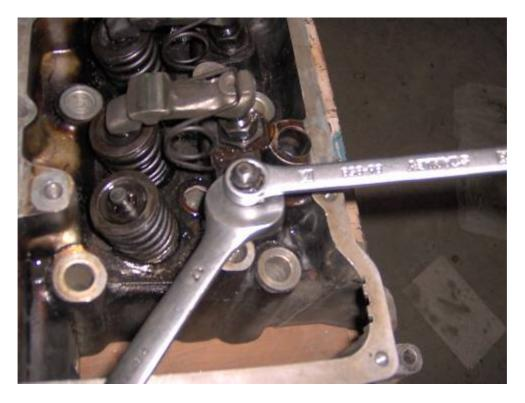
On the first article of this series I stressed the importance of storing valvetrain components coming from different locations separately. The key to avoid mixing up components from different valves is to remove each part one at a time, then toss them on a solvent bucket...
