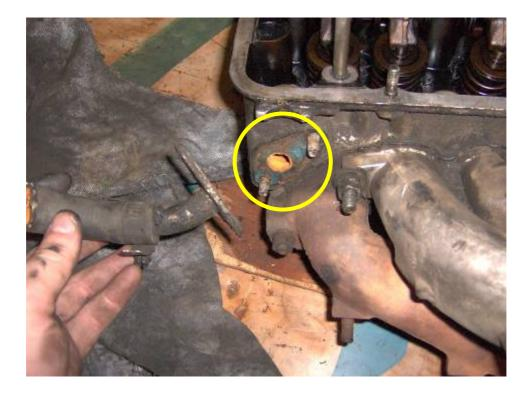
Use a long 13mm socket to loosen the nuts on the thermostat/upper radiator hose Tee connection and remove the latter from the head. That plugged-up short section of hose is where the thermostat is supposed to go, but I got rid of it a few years back since it's not needed in a 30° C+ year-round weather:
