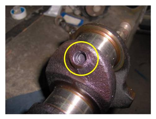
Nevertheless, the rear end of the crankshaft houses a small bearing (named pilot or spigot bearing) which should be replaced every time the engine or gearbox is removed regardless of its condition:
