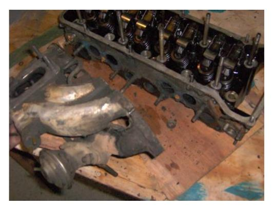
Use a small flathead screwdriver to pry out and remove the manifold gaskets:
