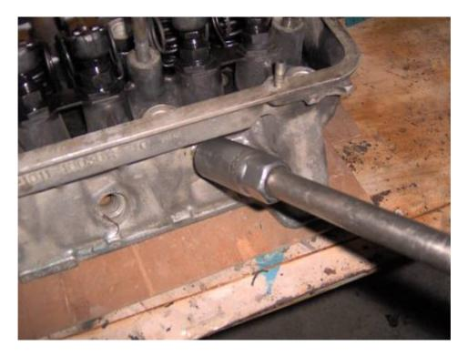
Although not mandatory, all work on the head will prove easier if all of the studs are removed first. The easiest way is by using a couple spanners to jam two nuts together on the stud threads and then using a spanner to drive the stud out like a conventional hex bolt. Head studs come in only two sizes (5mm and 8mm), so make sure you have two nuts of each size and two 10mm and 13mm spanners:
