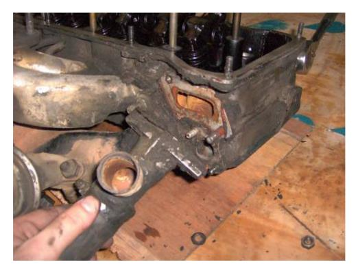
Use the long 13mm socket along with a 6" extension and the ratchet to remove the intake and exhaust manifold fastening nuts:
