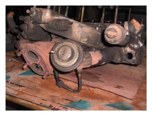
Start work by using a 10mm socket to loosen the timing chain damper fastening bolts. Once the damper is removed the head will sit level with the workbench:
