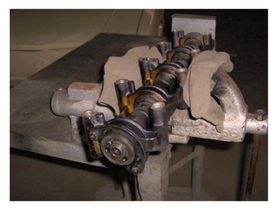
Use a 10mm spanner to loosen the camshaft thrust plate nuts (located at the front of the bearing housing) and then remove the camshaft thrust plate itself:
