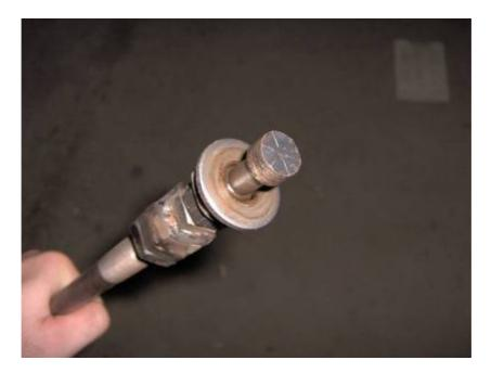
The picture shows how the improvised puller device is inserted through the bearing inner race. I had to tip the slide hammer a little bit so the step right under the rounded bolt head could "snag" on the inner race:
