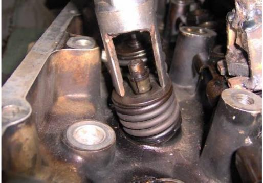
After compressing the springs, the collets can simply be removed using tweezers (I used a magnetic parts retriever for this purpose):
