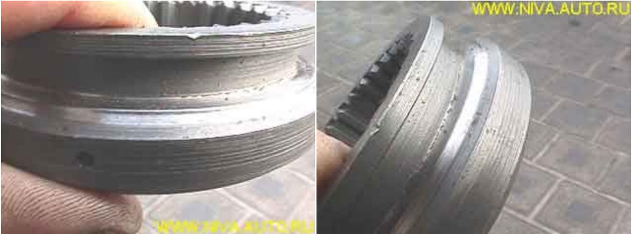
Check up that the gear hub splines don't jam on the sleeves, they should move freely in both directions:
