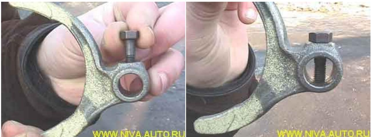
Insert the forks on the sleeves. They should move easily in circles:
