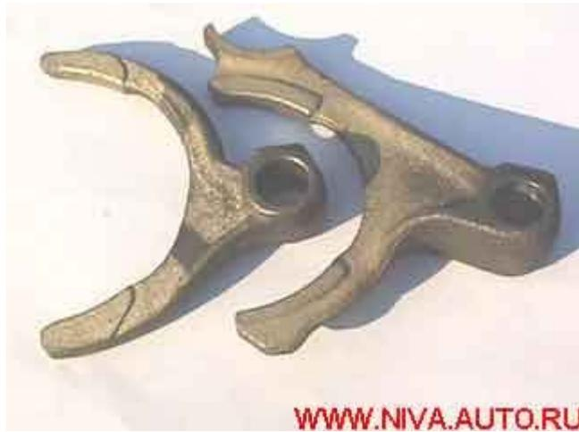
**The shift rails** should get into the fork holes with a little tightness. Check them by inserting each rail in its respective fork.
