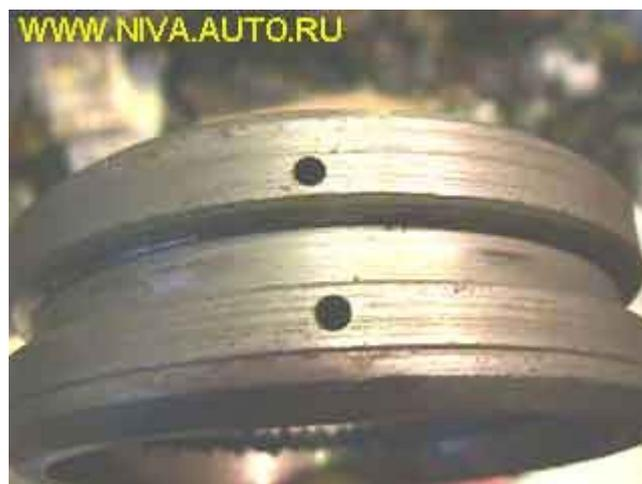
Some defective sleeves are shown below. On the left upper picture one channel is missing, on the right upper picture the channel is obviously displaced to the middle, and the bottom pictures show a badly chamfered sleeve:
