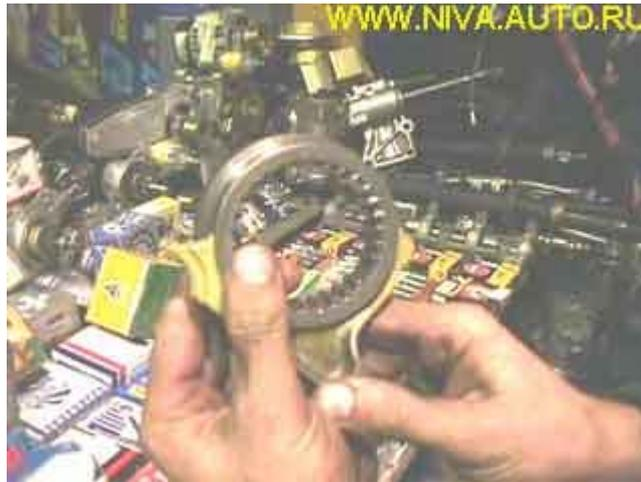
We've already described how to check the **hub splines**. The hubs of 1<sup>st</sup>-2<sup>nd</sup> and 3<sup>rd</sup>-4<sup>th</sup> speeds get damaged very seldom. The 5<sup>th</sup>-speed hub needs special attention, as it frequently jams on the sleeve:
