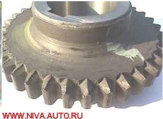
The gear cluster teeth and splines should be symmetrical and free of any damage:
