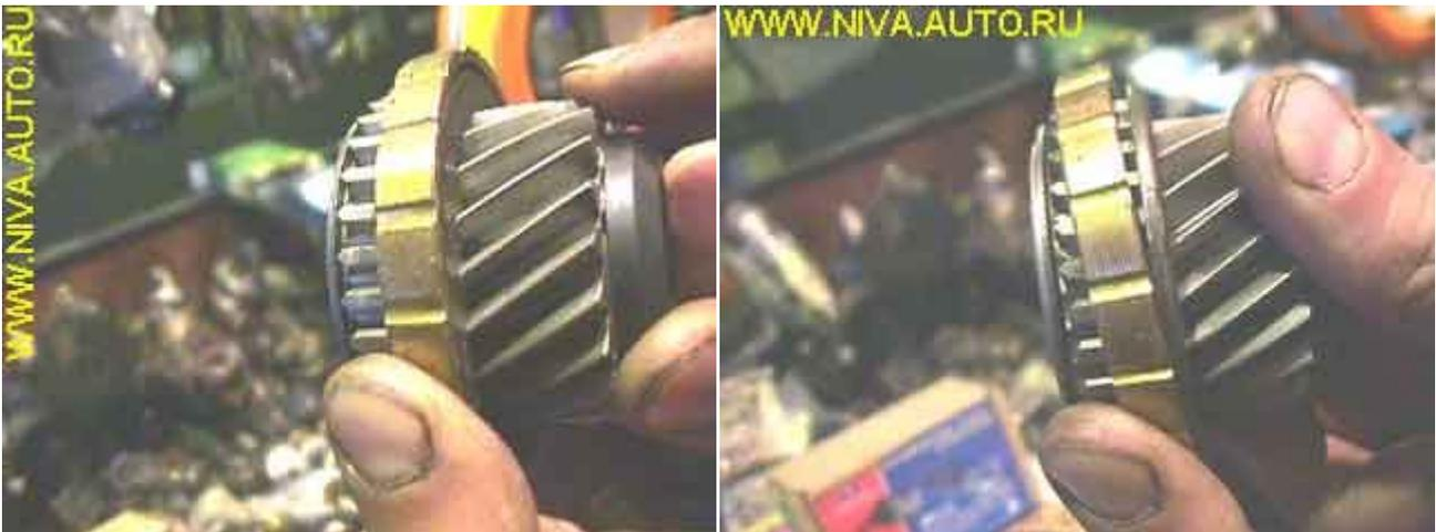
Grab the gear and synchronizer assembly and enclose it in the sleeve. Turn it a few times (left picture) and then push the gear into the sleeve, compressing the synchronizer spring (right picture):
