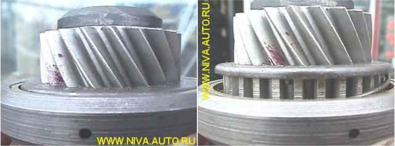
The 4<sup>th</sup>-speed gear is machined on the input shaft, but it's checked the same way as all others. The picture shows a 4<sup>th</sup>-speed gear with damaged straight teeth. This condition can't be seen in the picture, but note how the sleeve has jammed on the gear straight teeth and can't come back to its original position under the synchronizer spring action:
