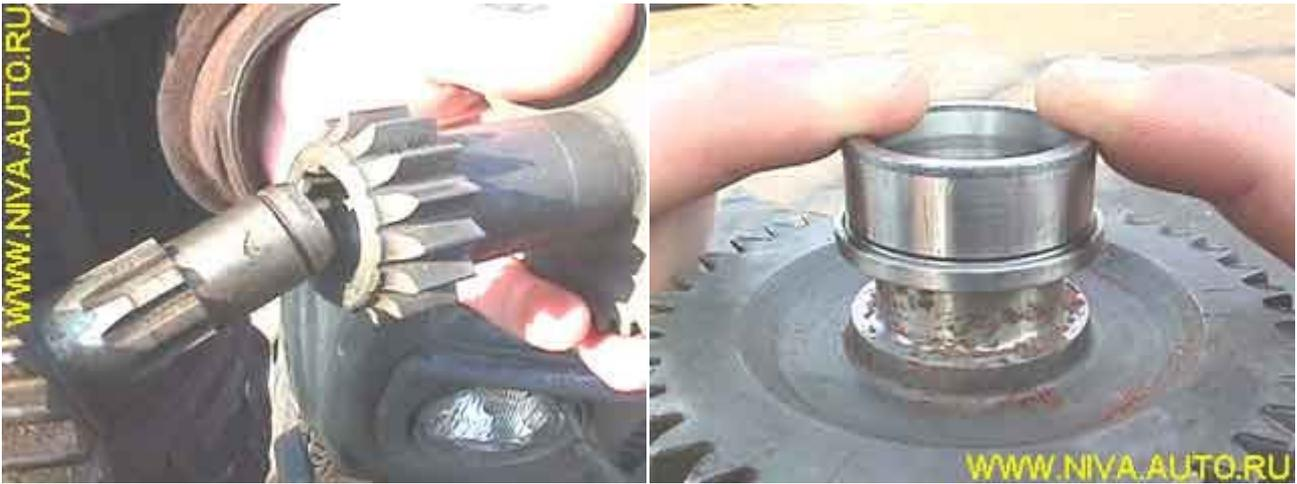
**The main shaft:** To check the shaft's diameter all gears, bushings, hubs, sleeves, bushes and bearings must be installed on it, on a new shaft all parts should go in with a small tightness. To check the splined end we must insert the rear flange and turn the shaft and flange in opposite directions and look for absence of play between both parts:
