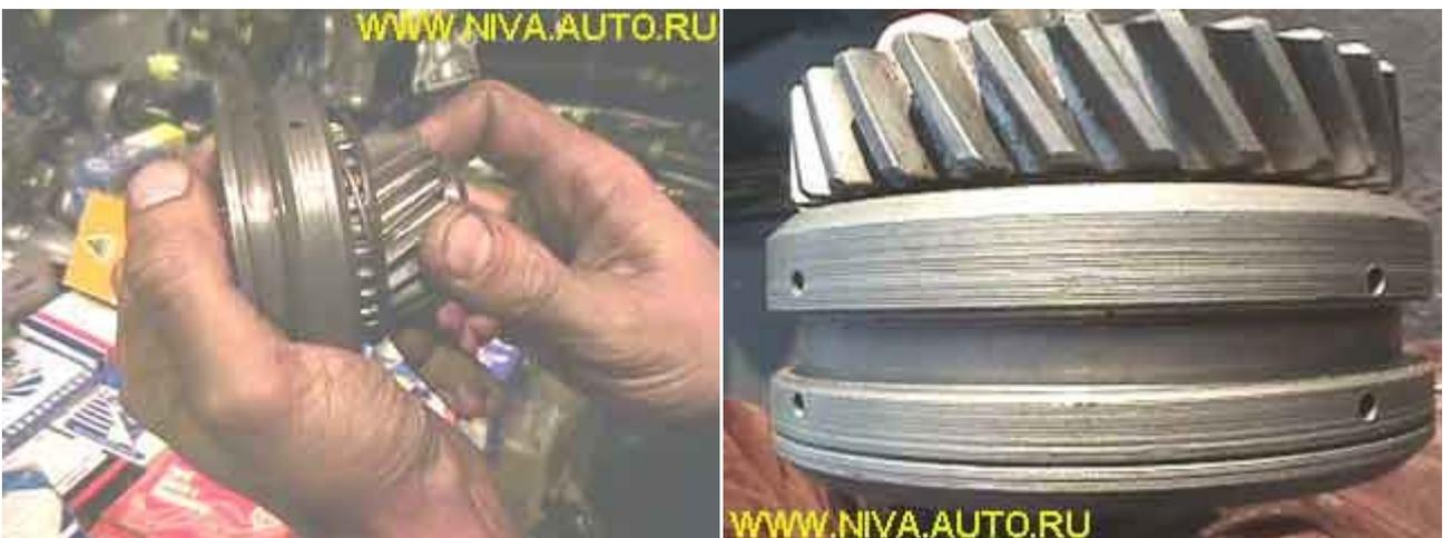
The gear should go on tight, but must enter and exit the sleeve easily without jamming. On the left picture it can be seen that the gear has jammed on the sleeve and can't return to the original position (right picture):
