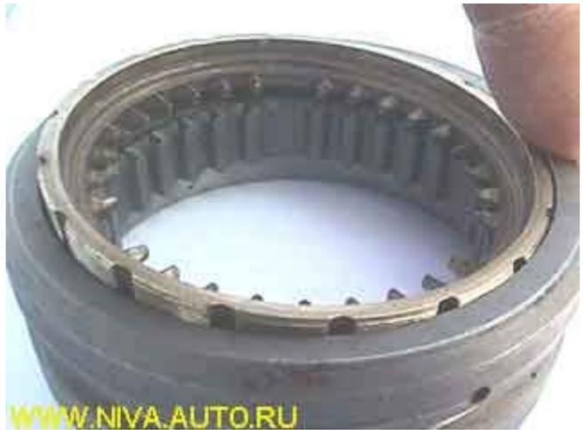
A normal synchronizer baulk ring shouldn't act strongly (below on the right an obviously bad synchronizer) and to be sunk in the sleeve more than 0.5 mm (at the upper right). The left picture shows a normal synchronizer baulk ring:
