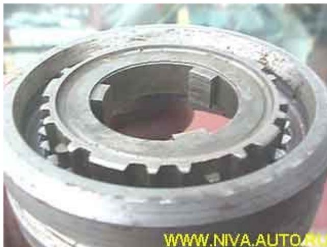
Check up that the sleeves are inserted easily on their gears (as is described above).
