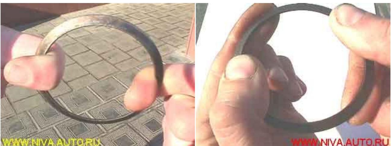
The spring washer must not be oval or distorted in any way:
