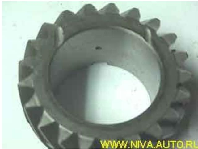
If it's necessary to buy **assembled gear/baulk ring sets**, check for absence of jamming between the baulk ring and the gear's straight teeth. Also check that the synchronizer spring sits squarely against the persistent ring. The synchronizer baulk ring must travel parallel all along the way, if it doesn't either the persistent ring is warped or the synchronizer's spring is incorrectly installed:
