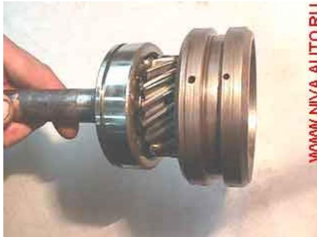
The splines of the input shaft must also be checked out. For this purpose insert the input shaft in the clutch disc and move the disc all the way up and down 2 - 3 times. The picture shows the disc has jammed on the input shaft end, which has gouged splines:
