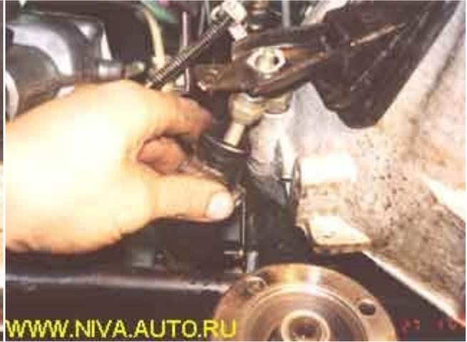
Use a long socket extension (or several short ones connected together) and a 13mm socket to remove the middle and bottom bolts of the starter. Shift the starter 1-2 cm towards the radiator:
