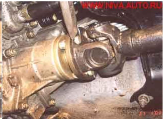
Disconnect the rear driveshaft from the transfer case. If the flanges are stuck together insert the chisel between them and strike 1-2 times with the hammer. Tie the driveshaft to the muffler:
