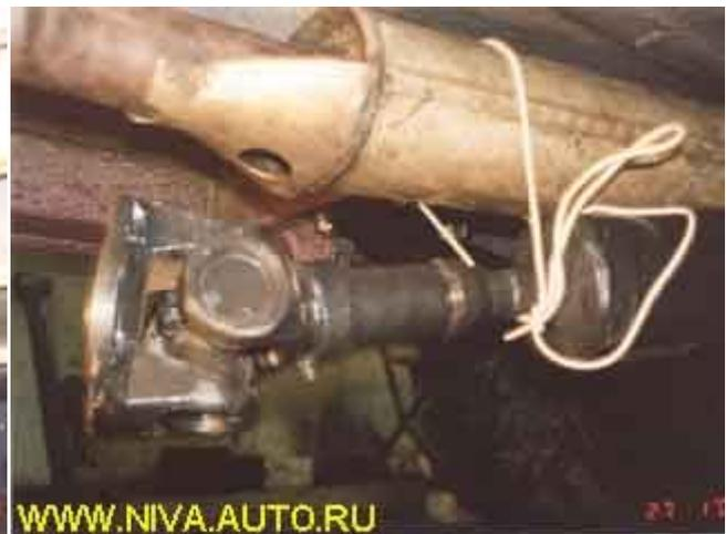
Remove the front driveshaft.
