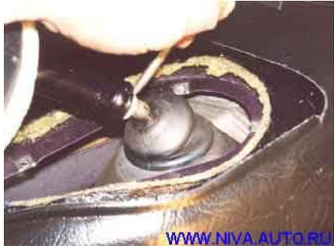
Remove the plastic retainer using four small screwdrivers to keep the tabs open, and then pull it out of the shifting mechanism extension:
