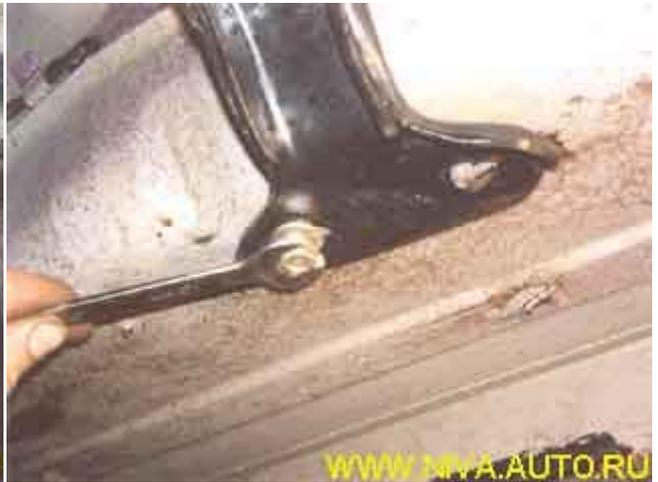
Remove 3 of the 4 engine-to-gearbox fastening bolts with a 19mm socket. To remove the top right one you'll need an extension piece of 1 – 1.2 m (see the right picture), then undo the top left bolt and finally the bottom right one:
