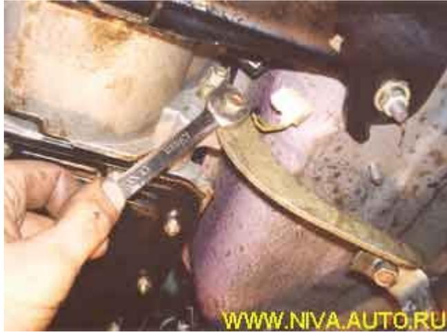
Use a 10mm wrench to remove two bolts of the front bellhousing cover and use a 13mm wrench to remove the four gearbox rear crossmember nuts:
