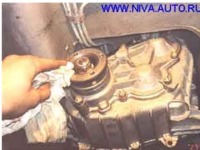
Reinstall the front and rear driveshafts using the alignment marks made earlier as a reference.
